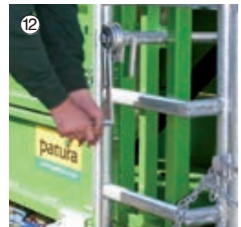
12 Recoilless hind foot winch for easy lifting the hind feet
