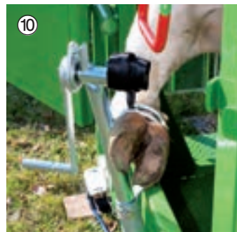
10 Recoilless front foot winch for easy lifting the front feet
