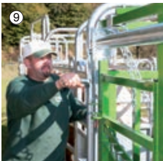
9 A comfortable belly strap winch for easy holding and release of the animals
