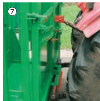
7 Transportable using linkage draw bar and upper link
