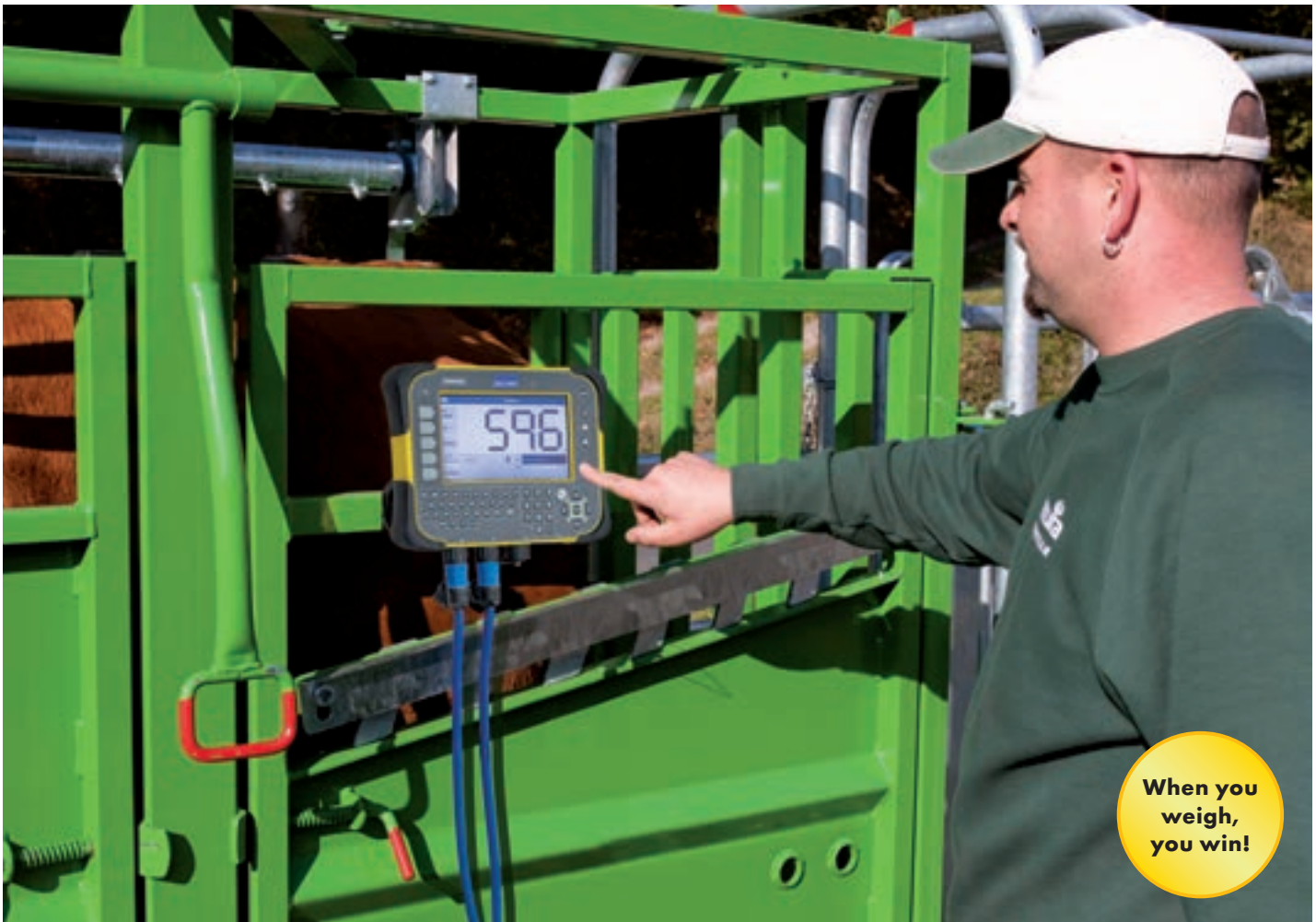
The PATURA cattle crush with the electronic Tru-Test scales, consisting of the indicator with digital display and 2 load bars (see "Weighing Systems")
