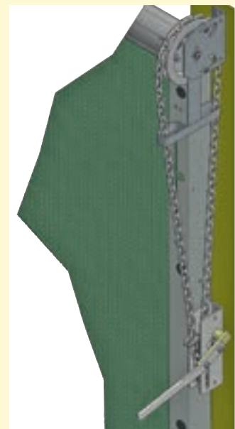
The fast, sturdy and easy-to-operate chain drive - 2 s/m
