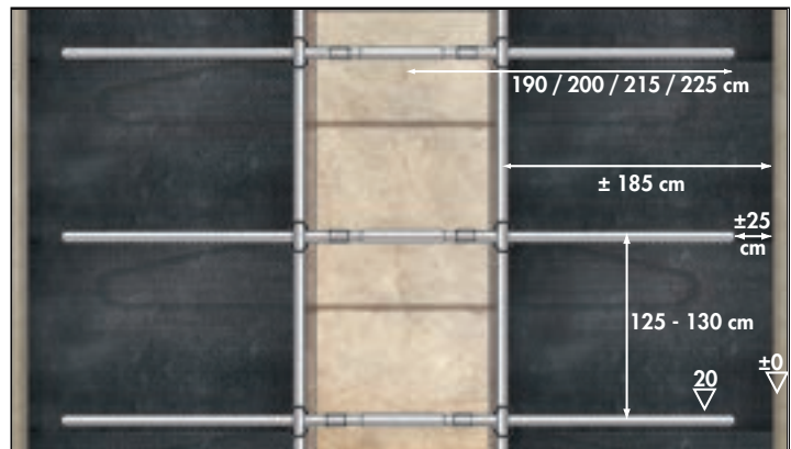
Variant 2: assembly dimensions for double row cubicle divider Universal on a floor mount bracket - for heavy livestock, example: high bed cubicle
