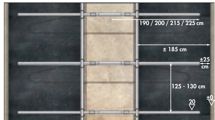
Plan view – assembly dimensions for double row cubicle divider Universal on a concrete raised box - for heavy livestock
