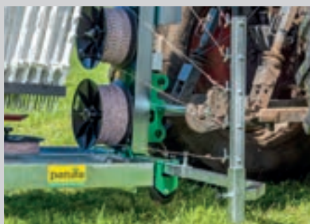
Up to 5 polywires and polytapes can be wound up or down in one run
