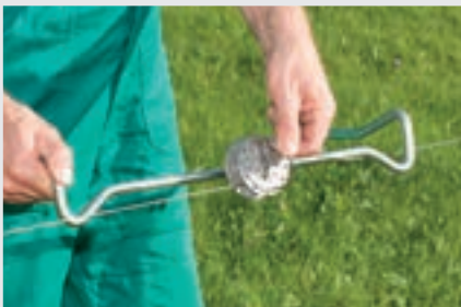
3. Hook the wire tensioner handle in the wire, install the cotter pin and remove the wire tensioner handle
