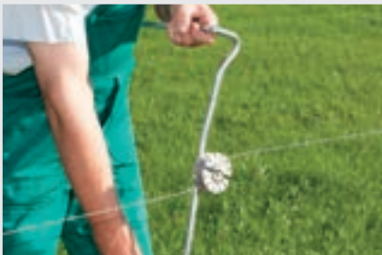
2. Turn the wire tensioner handle until the correct fence tension is reached
