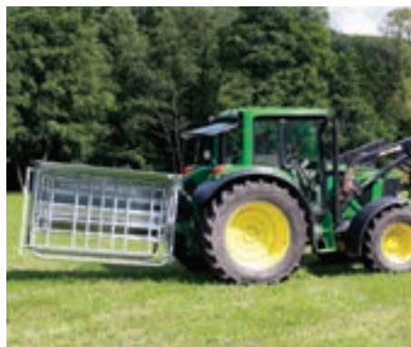
Transport via 3-point linkage with folded up calf creep enclosure
