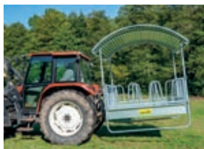
Transport using a 3-point linkage, up to 10 km/h when empty
