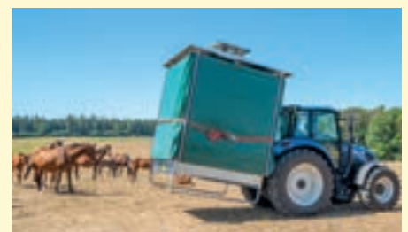
Transportation via 3-point linkage, when empty at max. 10 km/h, with down folded roof areas
