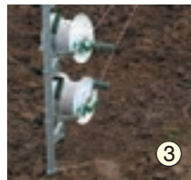
3 Grab the polywires from the reels and unwind
