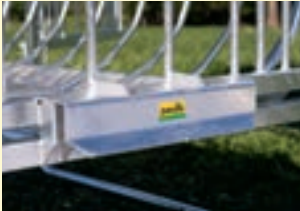
Solid linkage draw bar adapter for tractor draw bar
