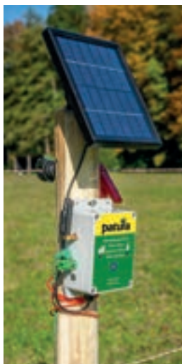
Place the GSM fence alarm at the end of the fence to ensure complete monitoring of your entire electric fence.
