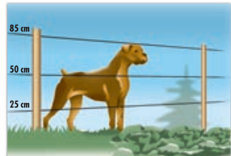
Electric fences for large dogs are 0.85 to 1.05 m high with 2 to 4 wires.
