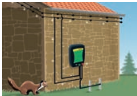
Electric fences for protecting against martens and raccoons consist of at least 2 wires that are placed close to each other and are connected alternately to the plus- and minus-pole of the device.
