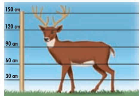
Electric fences for protecting against red deer are up to 1.50 m high with 5 wires.
