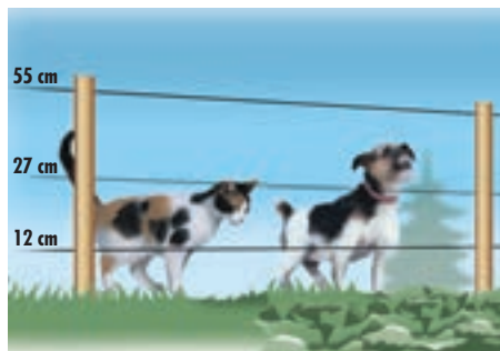
Electric fences for cats and small dogs are 0.55 to 0.75 m high with 3 to 4 wires.
