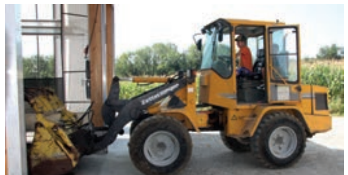
For efficient manure removal by loader, all box stall partition walls can fold away - each stall row is machine accessible along the entire length
