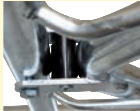
Internal plastic buffer for return of yoke
